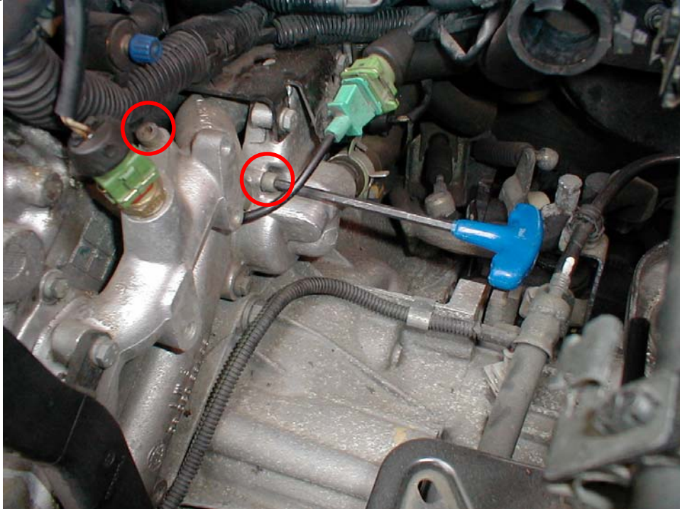
Fig 4: Thermostat housing bleed screws
