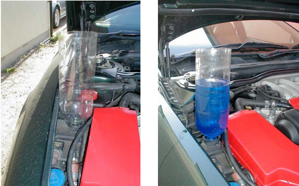
Fig 7 Finished header tank adaptor in place
